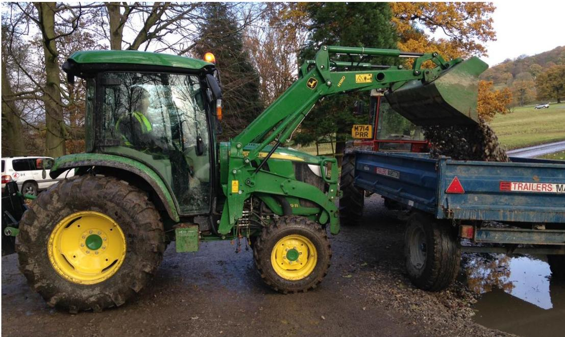
*Operating the John Deere H180 front-end loader. Picking up gravel in the bucket and depositing it in a trailer*
