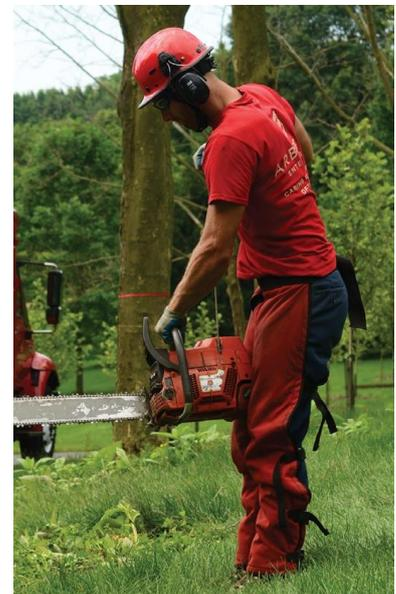
chain and throwing the brake on. If the brake does not work the chain should not be used and requires going off to an expert for repair. Since there are not many checks they have quickly become second nature to complete before beginning work with the saw.
